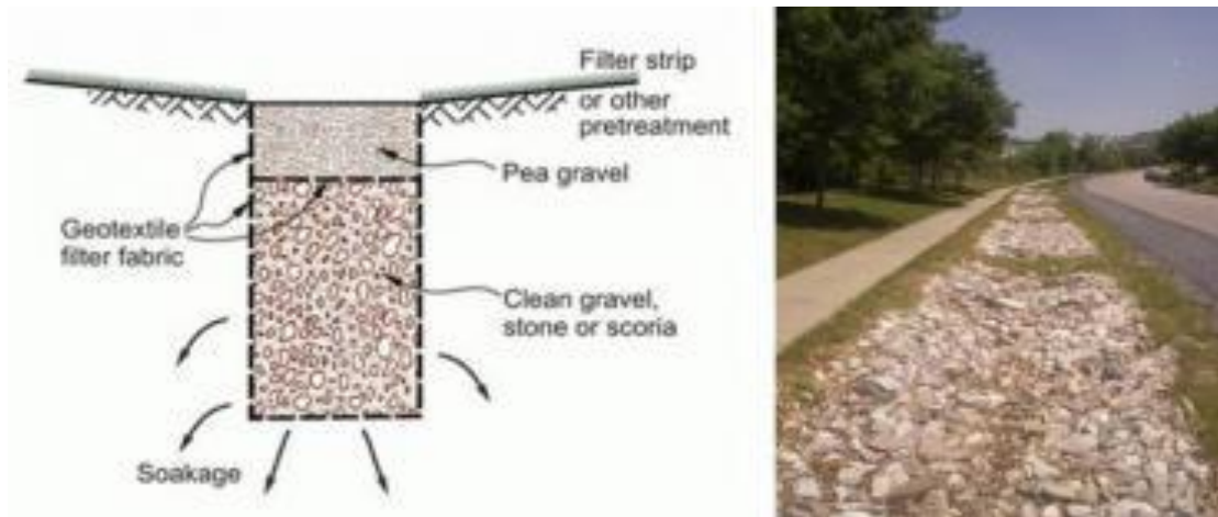
Figure VI-23 Infiltration trenches along the roadside to promote infiltration of runoffs
